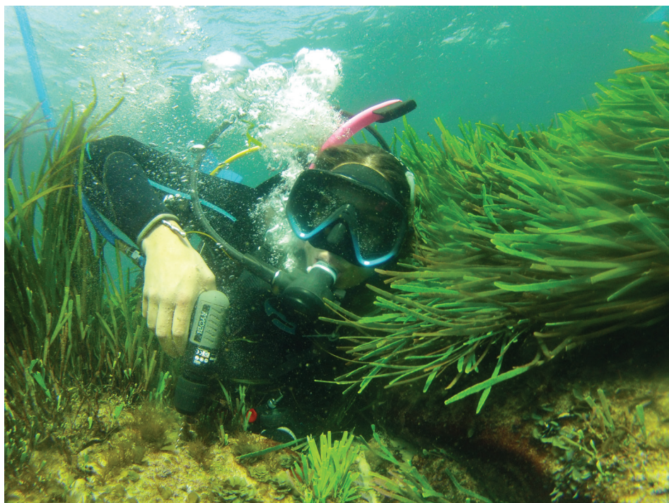
Dive officer Rochelle Johnston helps out with setting up an experiment in Wollongong. The blue hose connects the air drill to a scuba cylinder. Photo: Frederic Cadera, volunteer.
