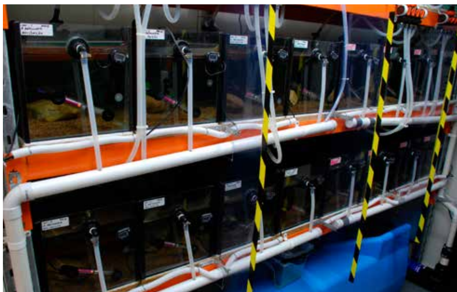
We use flow-through exposures (pictured here), as well as long-term mesocosm systems, to expose fish to environmentally realistic levels of contaminants of emerging concern.
