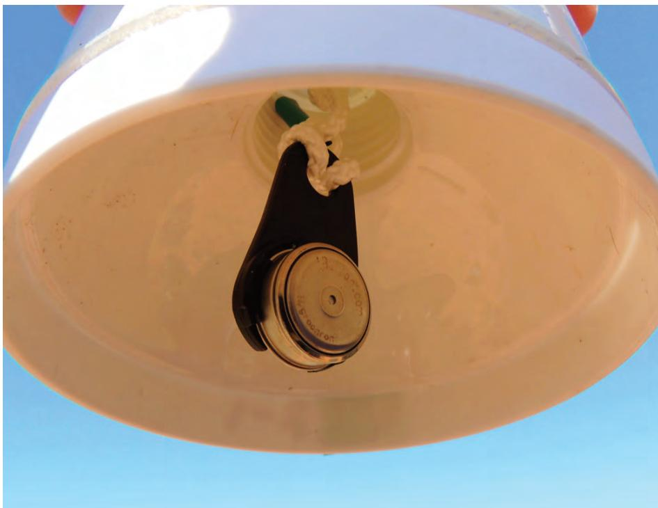
Small data logger unit with shading, ready to be placed out into the field (Photo: Andrea Leigh, 2013)
