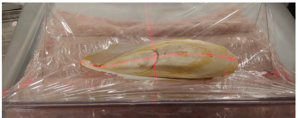
A Sepia apama cuttlebone about to be CT scanned. By using CT, James can accurately assess the density of a cuttlebone nondestructively, which is necessary when working with museum specimens.
