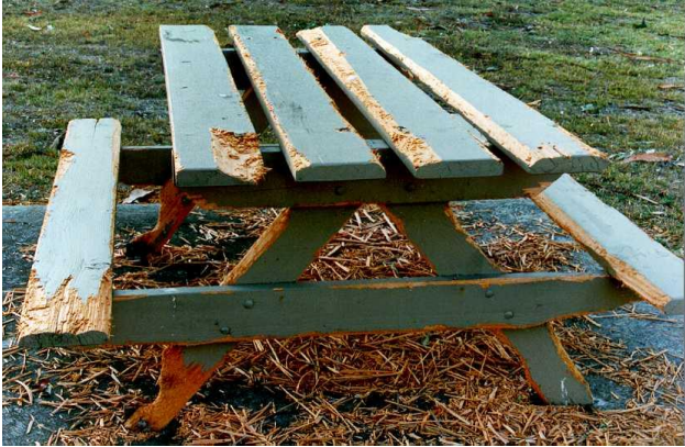
Figure 6: Cockatoo damage to outdoor furniture
