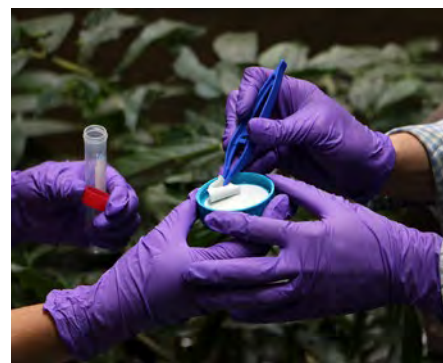
After pumping stream water through a filter to collect environmental DNA, genetic methods are used to assess the presence of both Batrachochytrium dendrobatidis and target frog species in the waterways. Image: Dr Laura Grogan.
